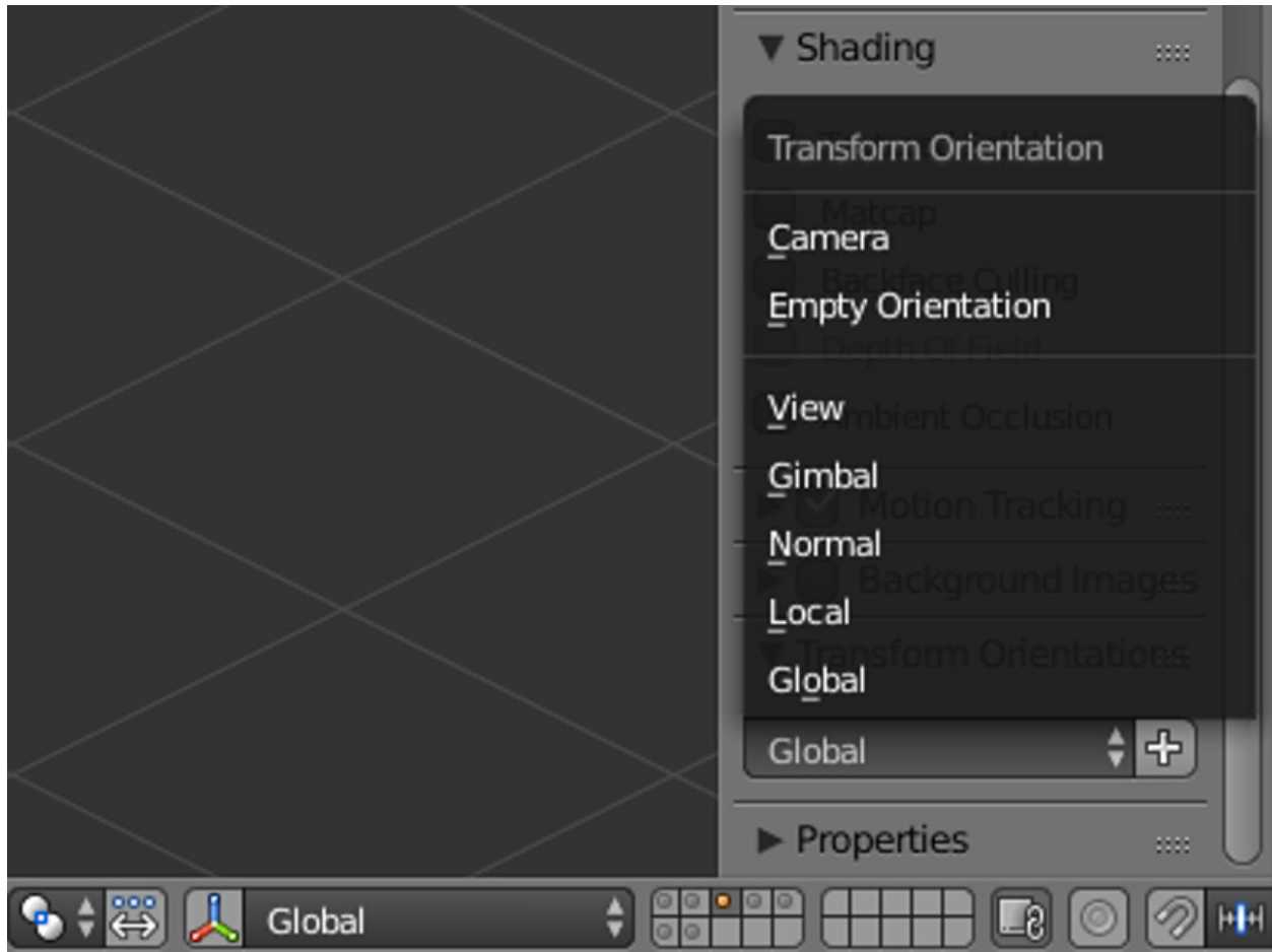
Fig. 23: The Transform Orientations of the current scene. All of these will be used by Align Tool except for Gimbal and Normal.
